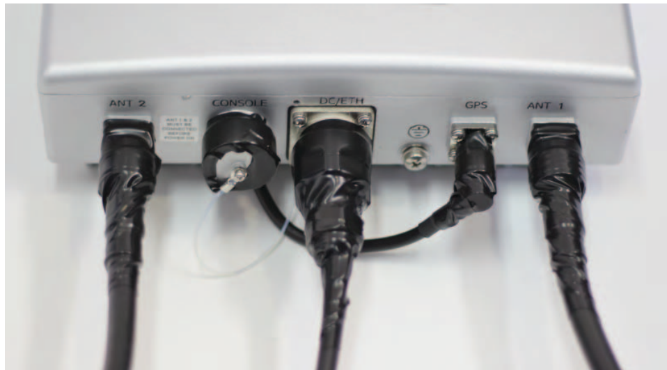
Figure 4.18. Base Station Connectors wrapped with Splicing and Electrical Tape
