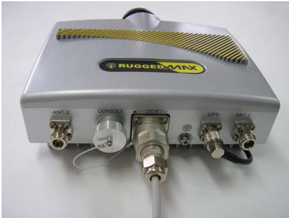
Figure 4.8. PoE connector secured to base station
