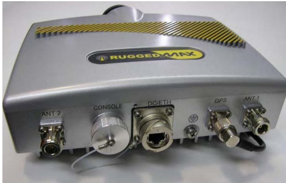
Figure 2.3. WiN7200 Small Form Factor Base Station Interface Panel
